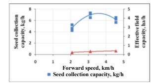
**Fig 4.** Relation between forward speed of operation, seed collection capacity of machine and effective field capacity in Dinanath grass
