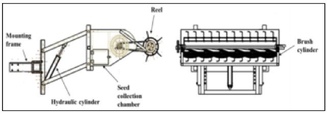
Fig 1. Plan and elevation of tractor operated grass seed harvester
