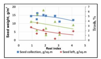
**Fig 5.** Relation among reel index and seed collected from unit area, seed left in the crop in unit area and trash coming in seed collection box during seed collection in Cenchrus grass
