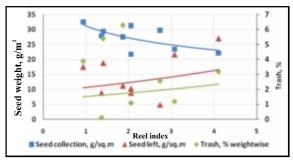
**Fig 3.** Relation between reel index and seed collected from unit rea, seed left in the crop in unit area and trash coming in seed collection box in Dinanath grass
