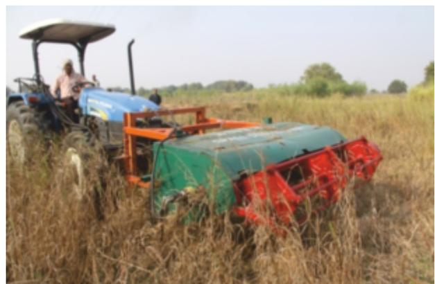
Fig 2. Operation of tractor operated grass seed harvester in Dinanath grass
