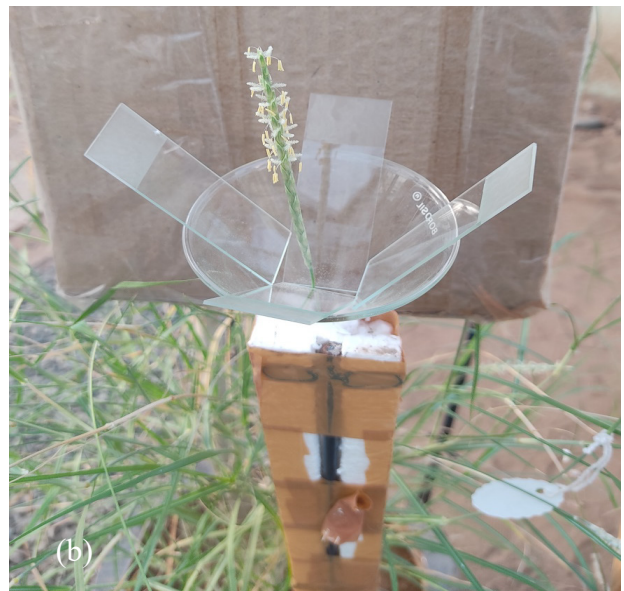
Fig 2. (a) Modified method of pollen count at different heights of spikes (b) individual funnel showing the arrangement of slides placed into it
